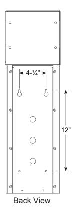
Secure the wall box to any flat surface using mounting hardware suitable for the surface you are mounting to. Top mounting holes are 4-1/4" apart and top to bottom mounting holes are 12" apart. There are 3 knockouts on the back and 2 underneath for routing wire.
