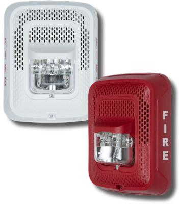
**The System Sensor L-Series** of speakers and speaker strobes reduce costly ground faults using a plug-in design and universal mounting plate that allow the installer to pre-wire mounting plates, dress the wires, and confirm wiring continuity before plugging in the speakers. In addition, a protective plastic cover prevents nicked wires by covering exposed speaker components.
