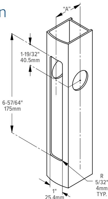
Adjustable mounting tube bracket may be removed for mounting on bridges, tabs, or other methods.
