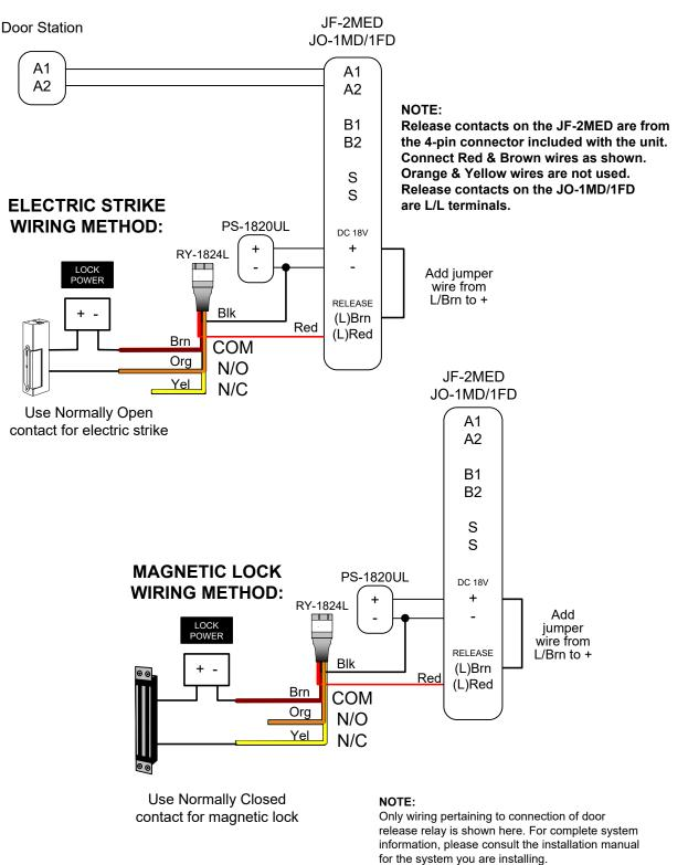
NOTE: The door release contacts on the station are rated at 24V AC/DC, 500mA. The RY-1824L should be used in any application where the strike or maglock has a higher voltage or draws more current. Otherwise, internal damage to the master station could occur.
