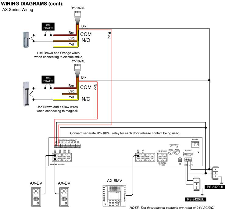
NOTE: The door release contacts are rated at 24V AC/DC, 500mA. The RY-1824L should be used in any application where the strike or maglock has a higher voltage or draws more current. Otherwise, internal damage to the Exchange Unit could occur.
