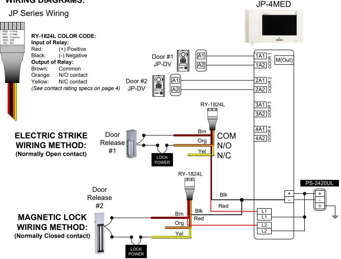
NOTE: The door release contacts on the station are rated at 24V AC/DC, 500mA. The RY-1824L should be used in any application where the strike or maglock has a higher voltage or draws more current. Otherwise, internal damage to the master station could occur.
