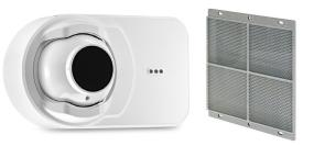
The OSI-RI-SK single-ended beam smoke detector is easy to install and adjust. Only the head unit needs to be wired, and the "eyeball" can be aimed without adjusting the detector mounting.
