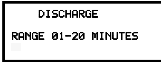
Pre-Discharge Setup Screen
