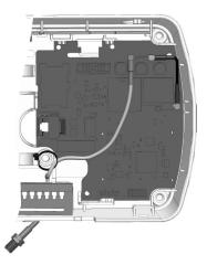
Figure 4: Installing the antenna connector
