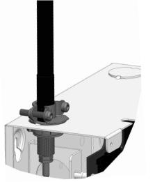
Figure 3: Antenna installation in a metal cabinet
