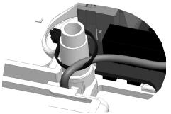
Figure 5: Securing the antenna connector
