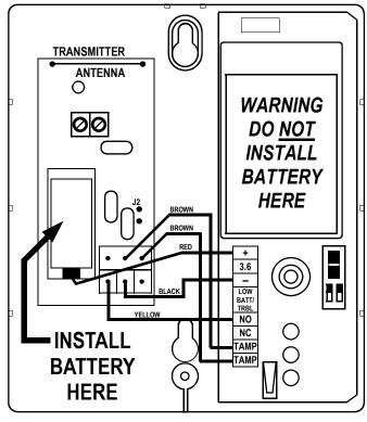
Fig. 2. GEMC-GB detector, front housing removed. Install battery in location shown.
