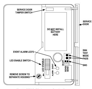
Fig. 1. GEMC-GB detector, Service Door open.
