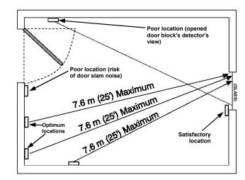
Fig. 3. Wall Mounting (Top View)
