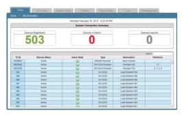
The EN6080-OP web browser home screen provides a snapshot view of end devices, including registered device, alarm and status information. From the home screen the following are available:
