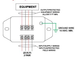
**DITEK's DTK-2LVLPF** is specifically designed to protect 24V SLC loops on fire alarm control panels where a current limiting feature is required. Its low-current fusing prevents induced surges from damaging sensitive (and expensive) control boards.
