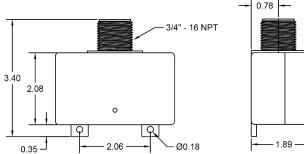
**DITEK's DTK-120HWLOK** surge protective device is designed and manufactured to meet the standards of the life safety industry. This compact, parallel-mount SPD is widely used to protect fire alarm panels and other dedicated branch circuit loads. It's small footprint enables installation in a variety of locations. The DTK-120HWLOK includes an NFPA 72 2013 10.6.5.2 compatible lockout kit to prevent accidental disconnect of the fire alarm system.
