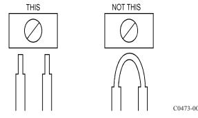
**FIGURE 5A. ACTIVATE TAMPER-RESIST FEATURE**
