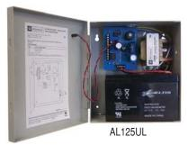
• AL125UL, AL125ULX, AL125ULP are Power Limited Power Supply/Chargers that will convert 115VAC 50/60Hz input, into two individually PTC protected 12VDC or 24VDC outputs (see specifications). They are intended for use in applications requiring UL Listing for Access Control (UL294) and applications requiring an interface with Fire Alarm Control Panels.
