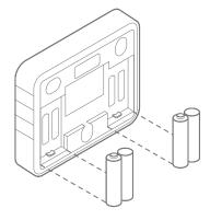
The thermostat can be powered by battery or 24 VAC. If a wall transformer is used to power the thermostat, connect between C and RH.
