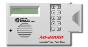
The AD-2000F dialer features busy-line and no-answer detection to ensure prompt transmission of up to 4 prerecorded messages delivered sequentially to as many as 8 standard telephones, cellular phones, voice and/or numeric pagers. Messages to both local and long-distance calls can be transmitted. When activated, the dialer instantly begins calling the numbers in sequence, delivering each message 1 to 3 times in a row, in accordance with the preselected number of dialing attempts.
