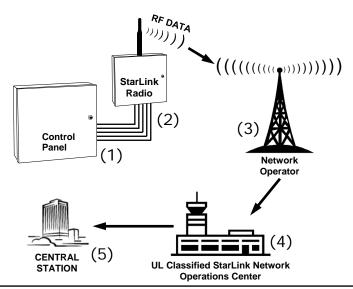
Center reports a trouble signal in the event that the network does not receive the expected supervision signal from the wireless communicator.
