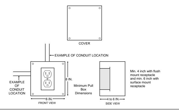
UL LISTED ELECTRICAL PULL BOX WITH LISTED OUTLET BOX AND NON-SWITCHED RECEPTACLE ON DEDICATED FIRE ALARM SYSTEM BRANCH CIRCUIT
