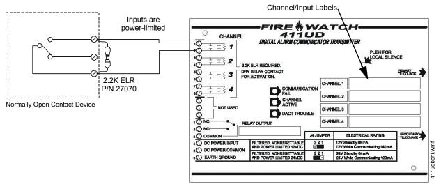
Figure 2.2 Style B Channel Connections
