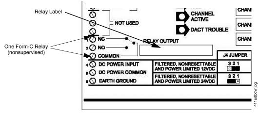
Figure 2.3 Programmable Relay
