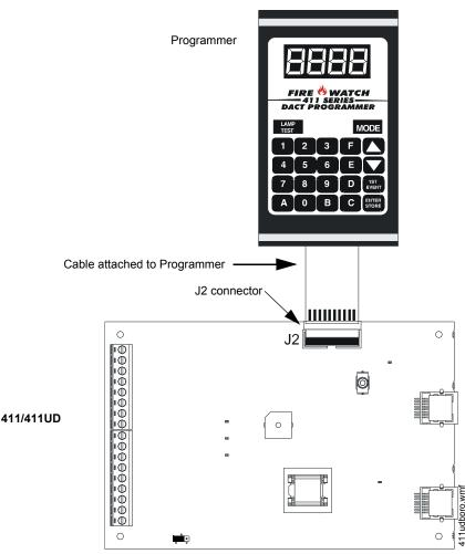
Figure 2.5 Programmer Connection to 411/411UD
