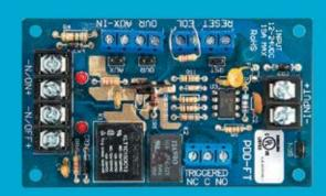
The PDB-1R uses an end-of-line resistor to trigger a form C contact in response to a fire system alarm condition.
