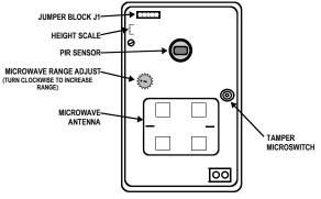
Fig. 4. Circuit board layout
