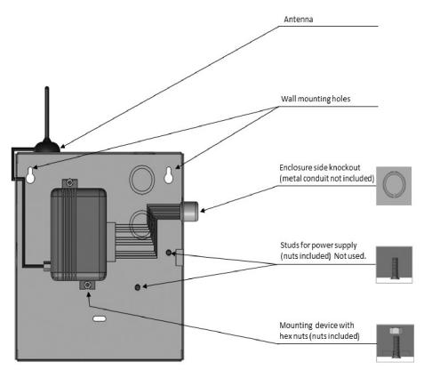
Figure 1: Mounting the Communicator
