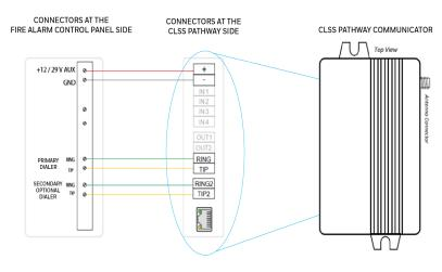
Figure 2: The Wiring Diagram
